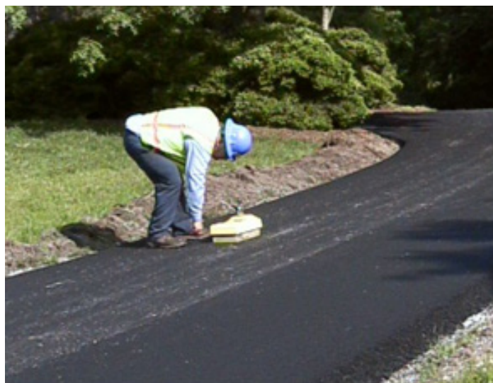
Measuring pavement density with a nuclear density gauge.
