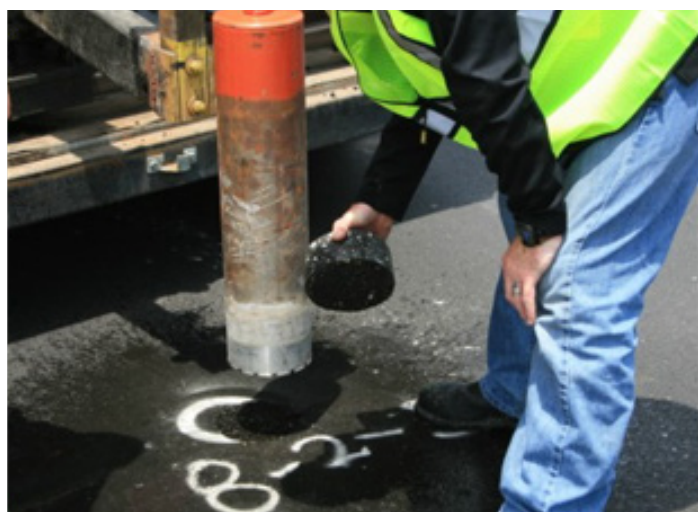
Coring an asphalt pavement.
