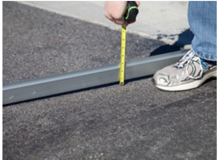
Measuring the rut depth of an asphalt pavement.
