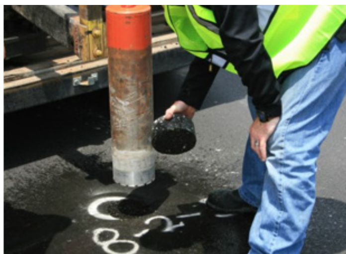
Coring an asphalt pavement.
