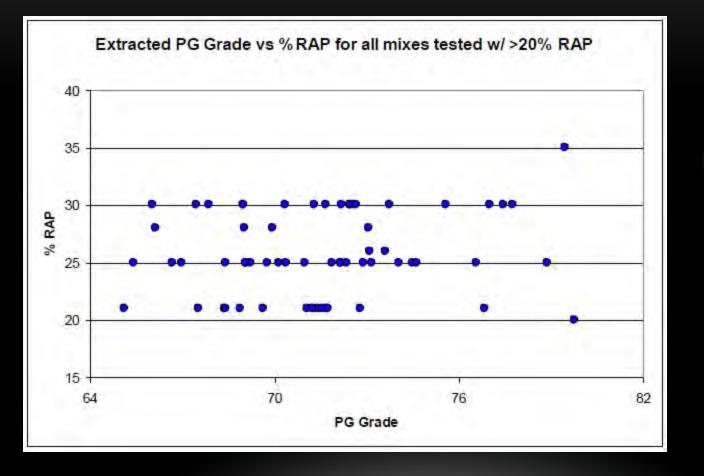
33/56 (59%) Mixes Graded Failed to Meet PG 70!
